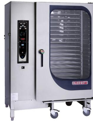
Combi's come in two basic designs. Boiler units with a built-in boiler tank that preheats and holds hot water to produce steam as needed, and boilerless units without holding tanks that spritz water directly onto the heating element to produce steam. Knowing which model is right for your operation can save you money and improve production right out of the gate.
